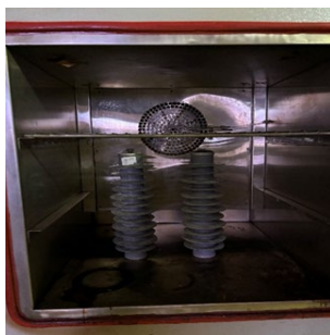
(a) MOSA kept on Oven for temperature
