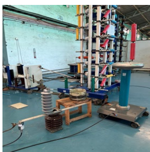
(b) Set-up for Impulse current application ageing at 150 °C
