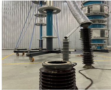
Fig. 3. Experimental set-up for PD measurement
