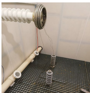
(c) MOSA kept inside salt-fog chamber
