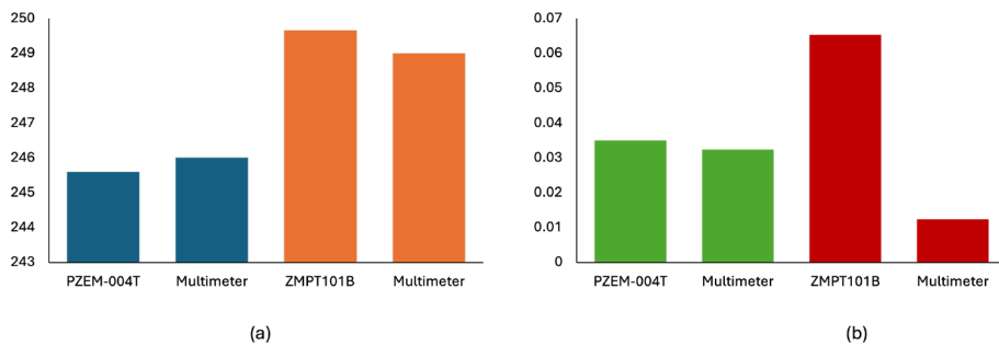
Figure 3. Measurement of (a) RMS voltage and (b) RMS Current at No-load
