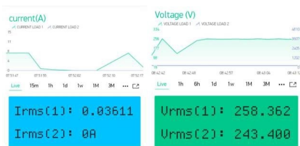
Figure 6. Graphical and real-time display for RMS current and RMS voltage of Load 1 and Load 2
