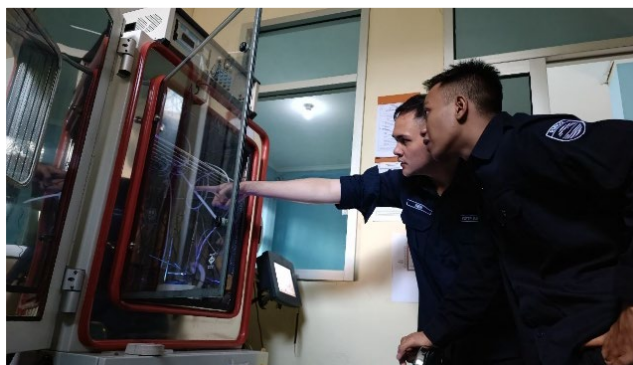
Figure 8. PT100 calibration process
